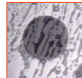
Above: Fingerprint oils on a connector end-face.
