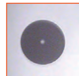
Below: A properly cleaned connector end-face
